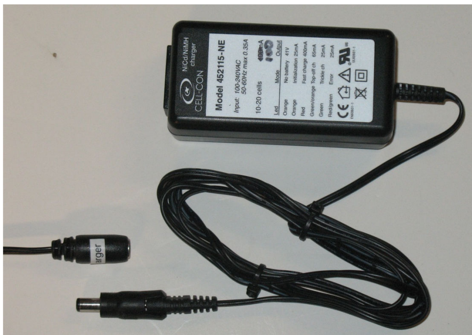
Figure 47. RibEye battery pack Cell-Con charger and battery cable charger receptacle
