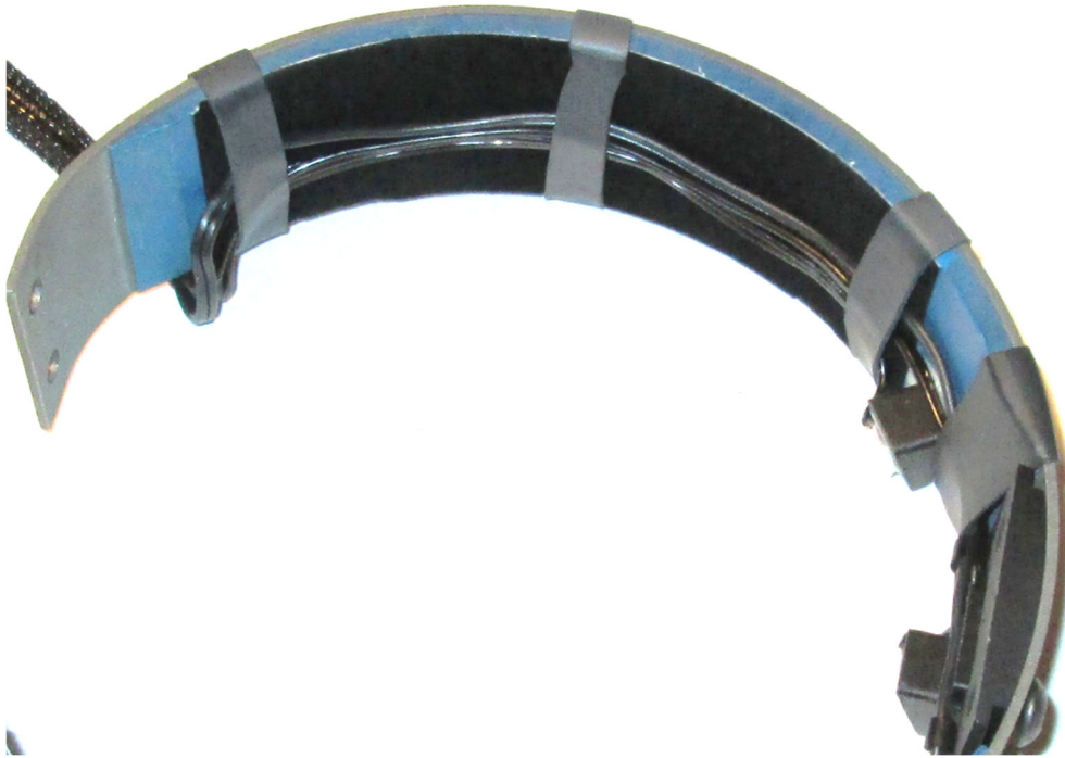
Figure 20. LED cables routed over flock paper
