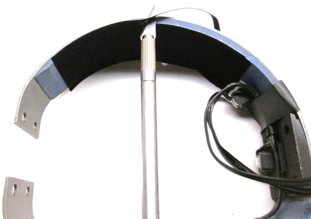
Figure 19. Excess flock paper being trimmed (view from edge of rib)
